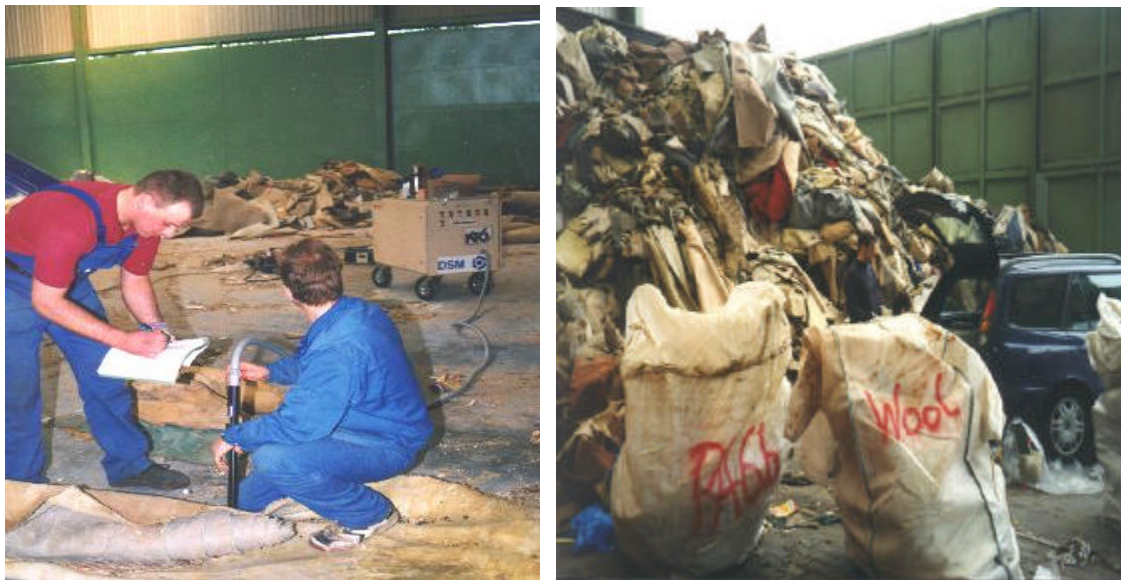
Figure 7. Manual sorting of waste carpets (left) and sorted material in big bags (right).
