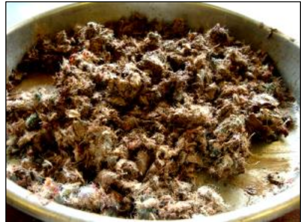
Figure 4. Mixture of fibre, soil and water
