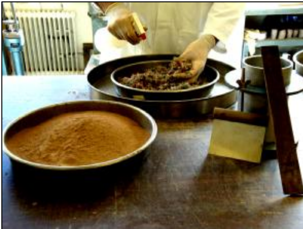
Figure 3. Mixing fibres with soil
