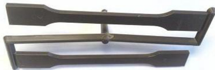
Test bars produced from post consumer PP carpet in trials
